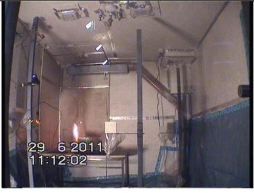
A video frame showing a laboratory setup with a fire source in the center. A smoke detector (RM7) is visible in the upper left corner. The timestamp is 29 6 2011 11:12:02. |
