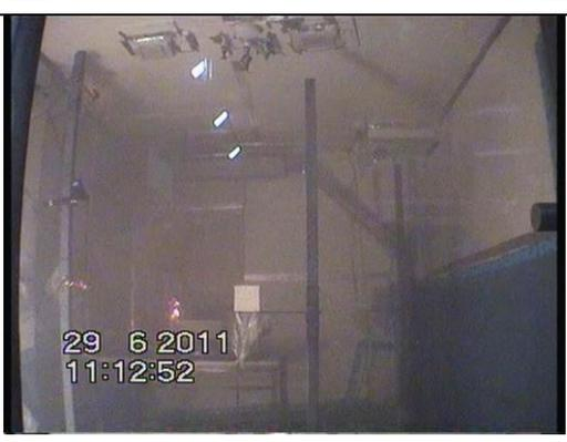
A video frame showing the fire source still active. A smoke detector (RM5) is visible in the upper right corner. The timestamp is 29 6 2011 11:12:52.                     |
