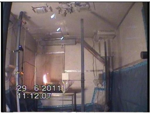
A video frame showing the fire source being extinguished. A significant amount of white water mist (ND-Wassernebel) is visible. The timestamp is 29 6 2011 11:12:07.        |
