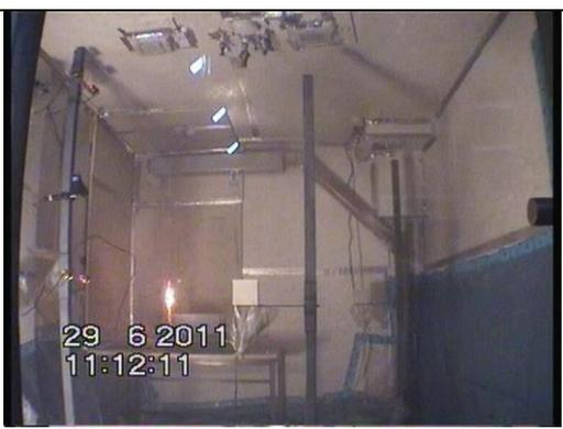
A video frame showing the fire source still active. A smoke detector (RM6) is visible in the upper left corner. The timestamp is 29 6 2011 11:12:11.                       |
